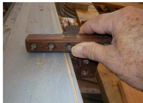
Above left Micky M is marking off some timber whilst making a set of pads to fit under our 'hollow' thwarts. Ian P and Steve B have reached a sticky stage in laminating as they walk a glued up plank round to the boat for Hamo T and Mike S to get to work. Above right the hand of Fred is using his scratch block to cut a tiddly piped edge to the inside of the starboard gunwale capping.
