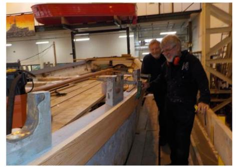
Above left Igor O, Hamo T, Mike F and Jeremy C are trying to remove the stubborn stem bolts. In the middle photo above John B is checking the position of the starboard rowlock crutches and over right Steve B and Ian P have made a start on fitting the outstanding sections of the port rubbing strake. This is the first section of lamination going in place.
