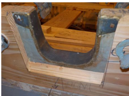
See above left with the poppet cutout nicely bevelled all round to give a secure home for the poppet. In the centre Mike S is doing the final fit on the starboard crutches. Far right Micky M is turning the last thwart stanchions after a couple of weeks practice. It obviously all paid off because at the top of the next page he is proudly presenting his finished article to Fred so that he could check it out. Obviously the 'Man from Del Monte' he say 'yes' judging by the relief on Micky's face
